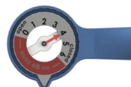
Figure 4: The compass of the eyeWatch Pen with the different positions available. '0' defines the fully open position where the outflow is not restricted when '6' is the fully closed position where the eyeWatch is maximally restricting the outflow. A movement counterclockwise decreases the fluidic resistance (6 towards 0) or clockwise increases the fluidic resistance (0 towards 6).
